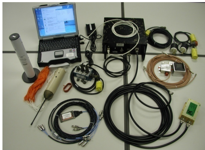
Figure 6. Panasonic Toughbook, Dropsonde (with chute), Interface Processor and Connections (Benney 2005)
